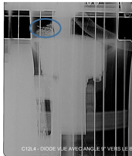
Fig.1 X-rays of the diode lead at the level of the half-moon connection for magnet C12L4, showing the presence of metallic debris.
