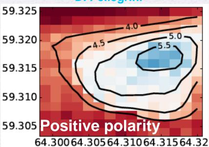
TuneScan\_LHCb\_off; Min DA;  $\beta^*$  =40 cm;  $\epsilon$ =2  $\mu$ m; I=1.15  $10^{11}$  e; Q'=15; I $_{MO}$ =500 A; X=140  $\mu$ rad.
