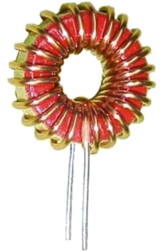
Powder core (compatibility with cryogenic temperatures unclear)
