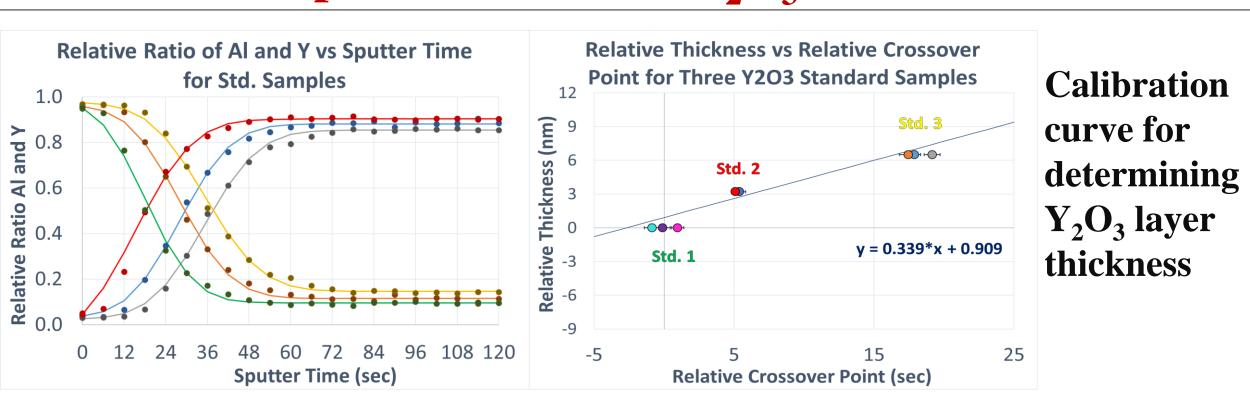
Three standard samples with known  $Y_2O_3$  layer thicknesses were sputtered to determine their crossover points. We then created a calibration curve by plotting the known thicknesses against their
