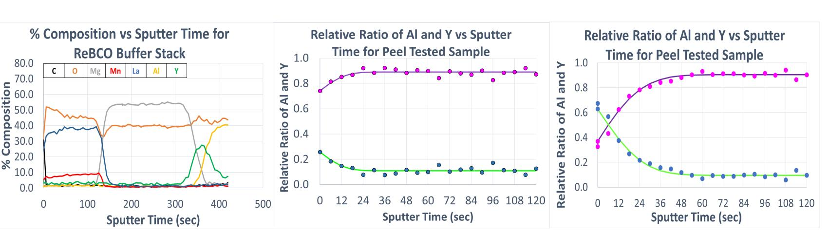
Composition data with sputtering depth (x) fit with the Gaussian Error (ERF) function.
