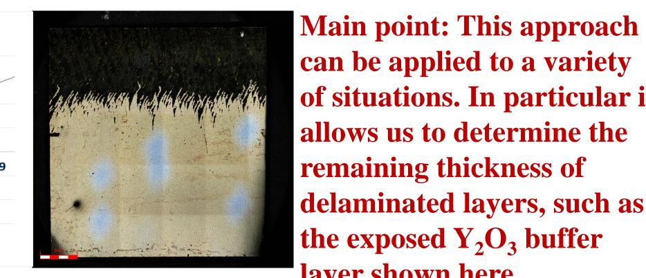
can be applied to a variety of situations. In particular it allows us to determine the remaining thickness of delaminated layers, such as the exposed Y<sub>2</sub>O<sub>3</sub> buffer layer shown here.
