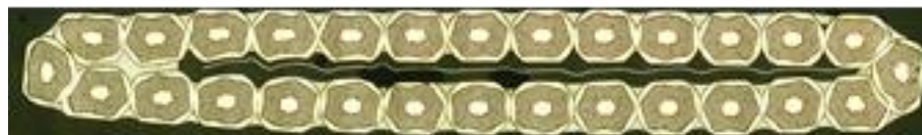
1 mm RRP150/169 28-strand cable with SS core
