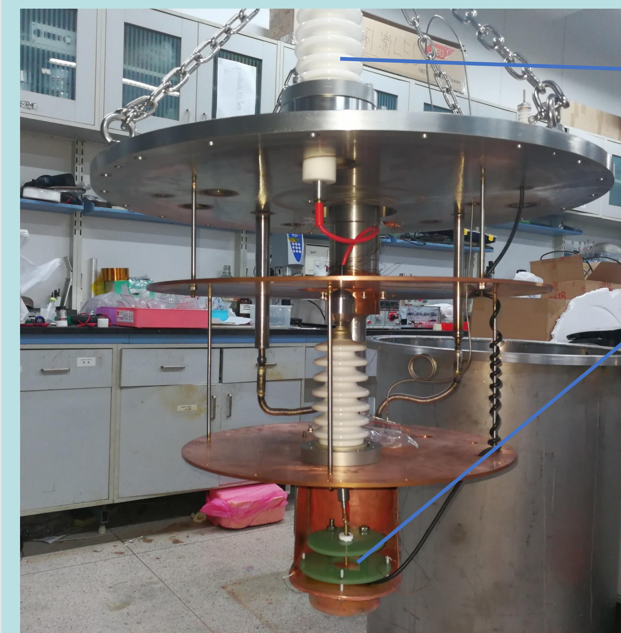
The internal structure of the cryostat on one side. The photo shows the electrical part in the cryostat. This part should be well insulated and it is used for test the sample dielectric performance.
