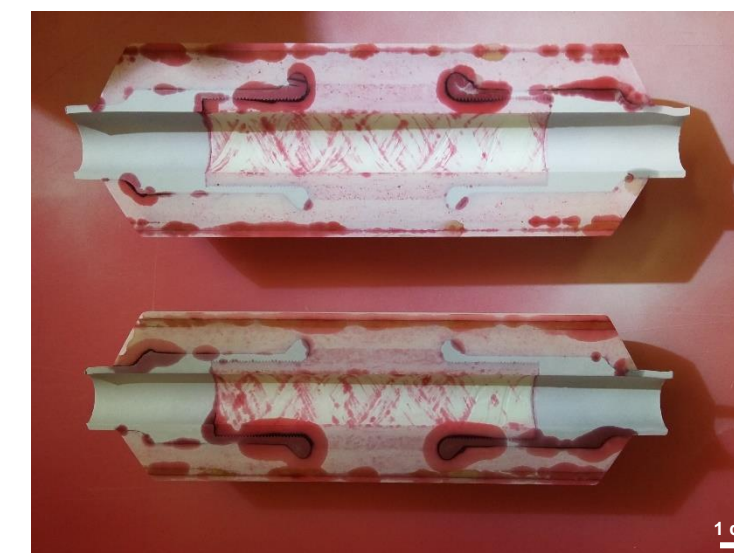
← Pronounced indications observed after PT for IBDH109. They are mainly located at the SS to composite interfaces, and in the GKG insulation layers
