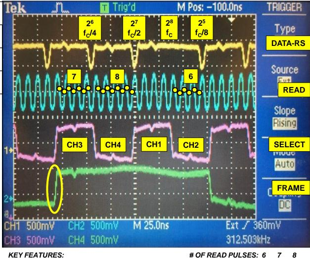
CIRCULATING ORDER CH1,CH2,CH3,CH4 FRAME PULSE AT THE BEGINNING OF CH3 # OF READ PULSES: 6 7 8 STORED NUMBER:  $2^5$   $2^6$   $2^7$ DATA RATE:  $f_c/8$   $f_c/4$   $f_c/2$
