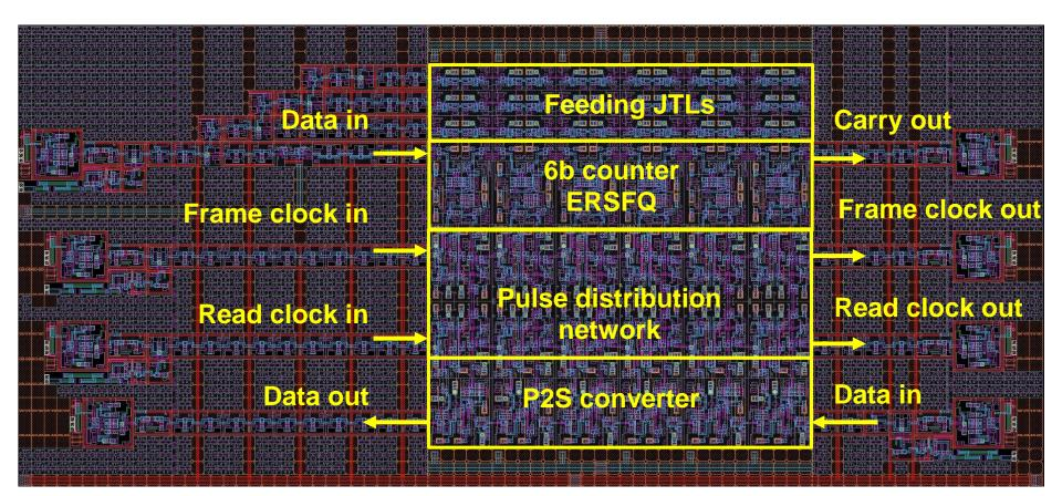
ERSFQ counter is 22.5 times smaller in area by converting to SFQ5EE
