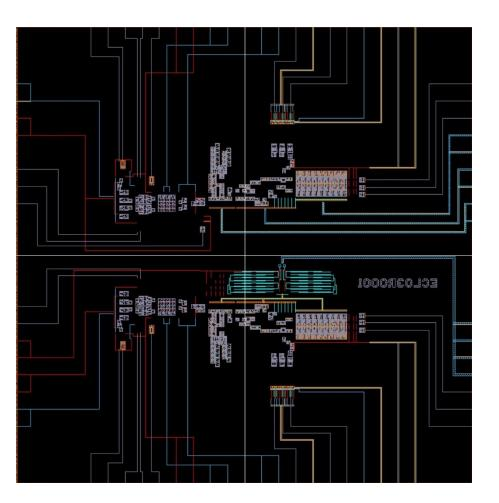
2 readouts (ERSFQ and RSFQ) are placed on the same chip
