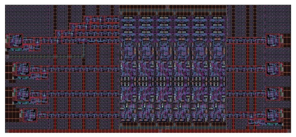
We designed both RSFQ and ERSFQ 6-bit counters using MIT/LL SFQ5EE process
