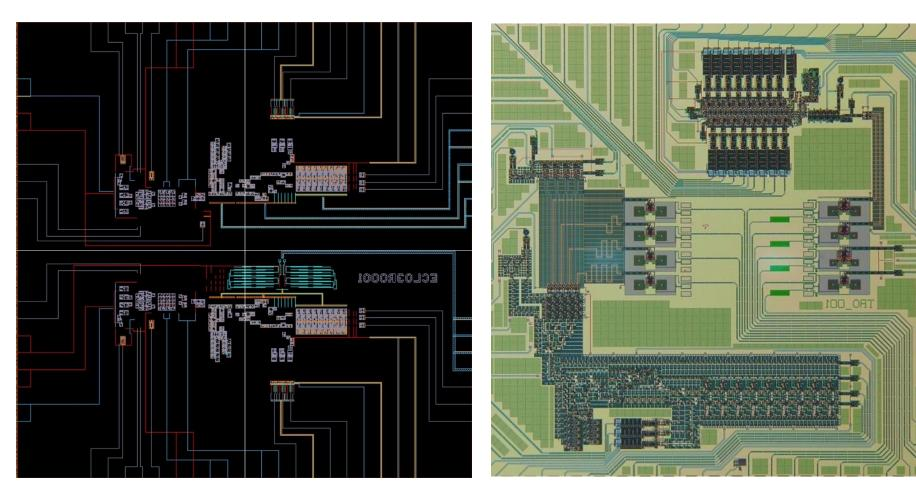
2 readouts (ERSFQ and RSFQ) are placed on the same chip
