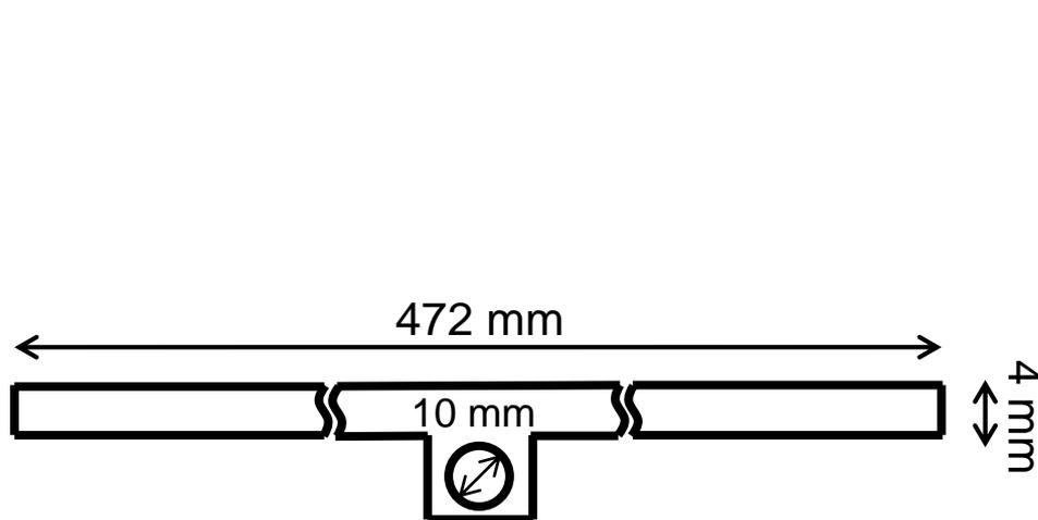
Fig.: Dimensions of one Al1050A cooling panel
