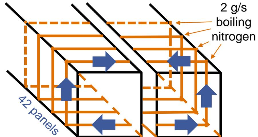
Fig.: Arrangement of the cooling panels around the detector
