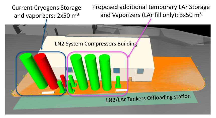
LN2 Storage Tank and Vaporizer (1x50 m<sup>3</sup>) LAr Storage Tanks and Vaporizers (4x50m<sup>3</sup>)
