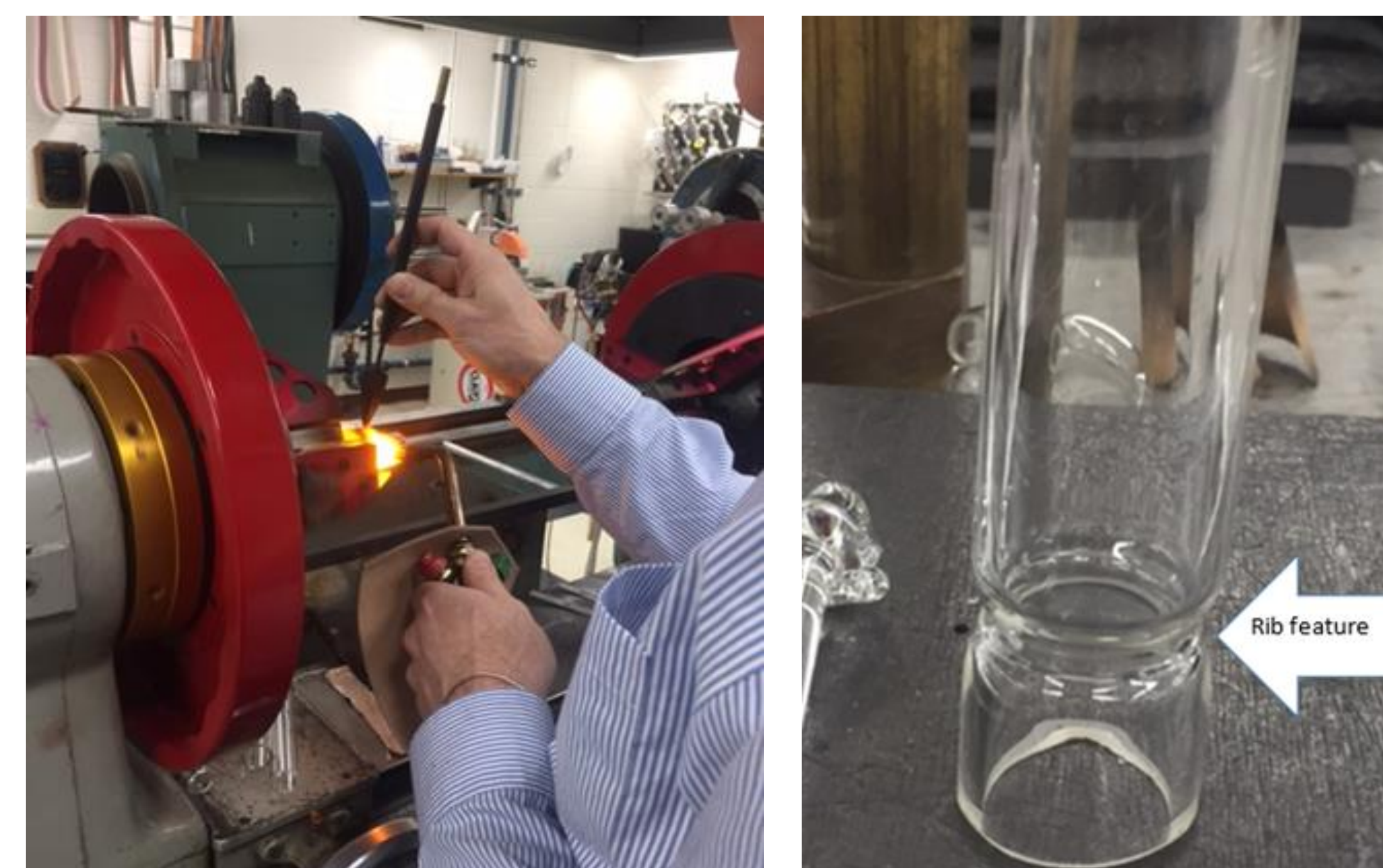
A rib feature making process is being presented by the glass blower. The rib separates the regenerator and the pulse-tube
