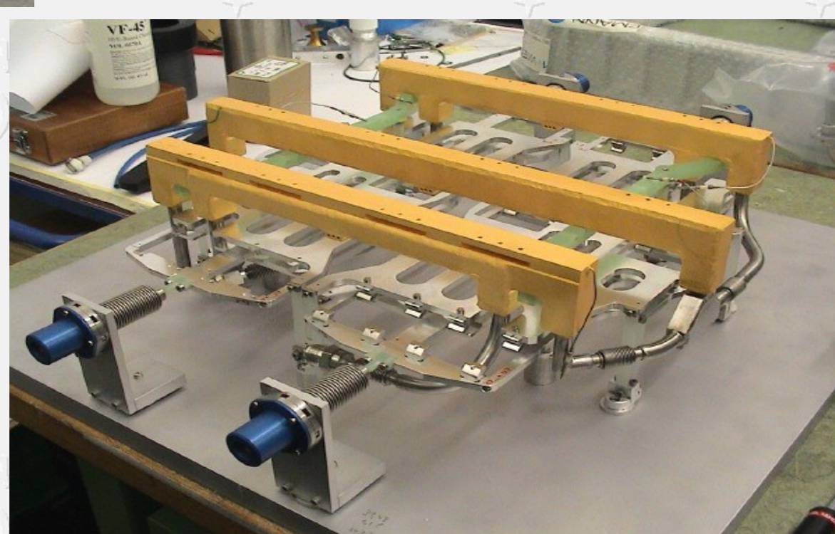
View of the heat exchanger in position on the top of the LN2 tank
