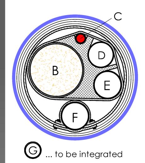
C The options 2) and 3) require an additional header at cryogenic temperature level, has to be in the integrated cryogenic distribuline without increasing its diameter.
