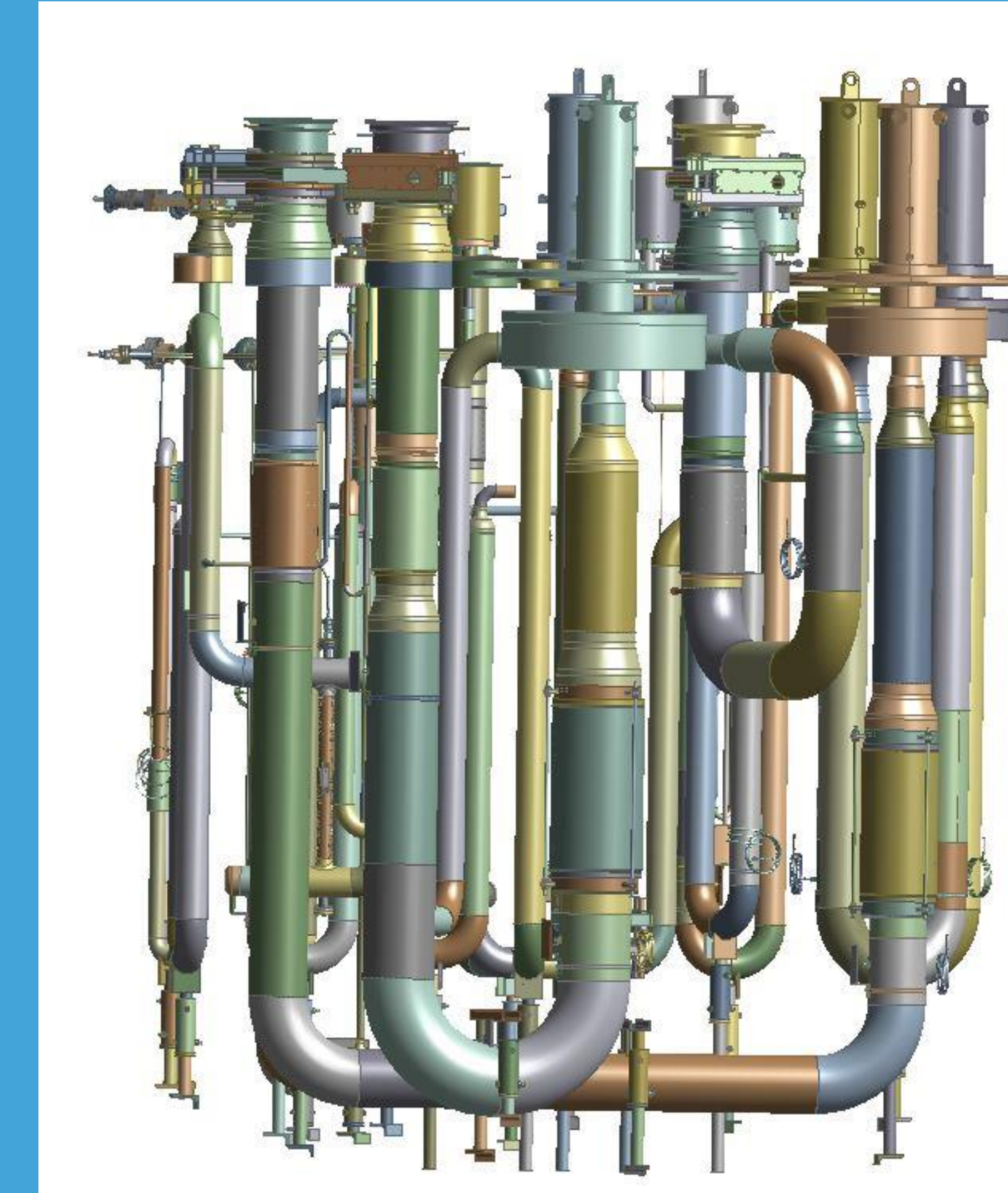
Fig. 2 Internal piping of cold box. All piping is designed in accordance with ASME B31.3-2014 Process Piping and local requirements. These local requirements include CBC, ASCE 7-10, and the Cryogenic Plant Seismic Design Criteria. AutoPIPE is used to perform flexibility analysis.
