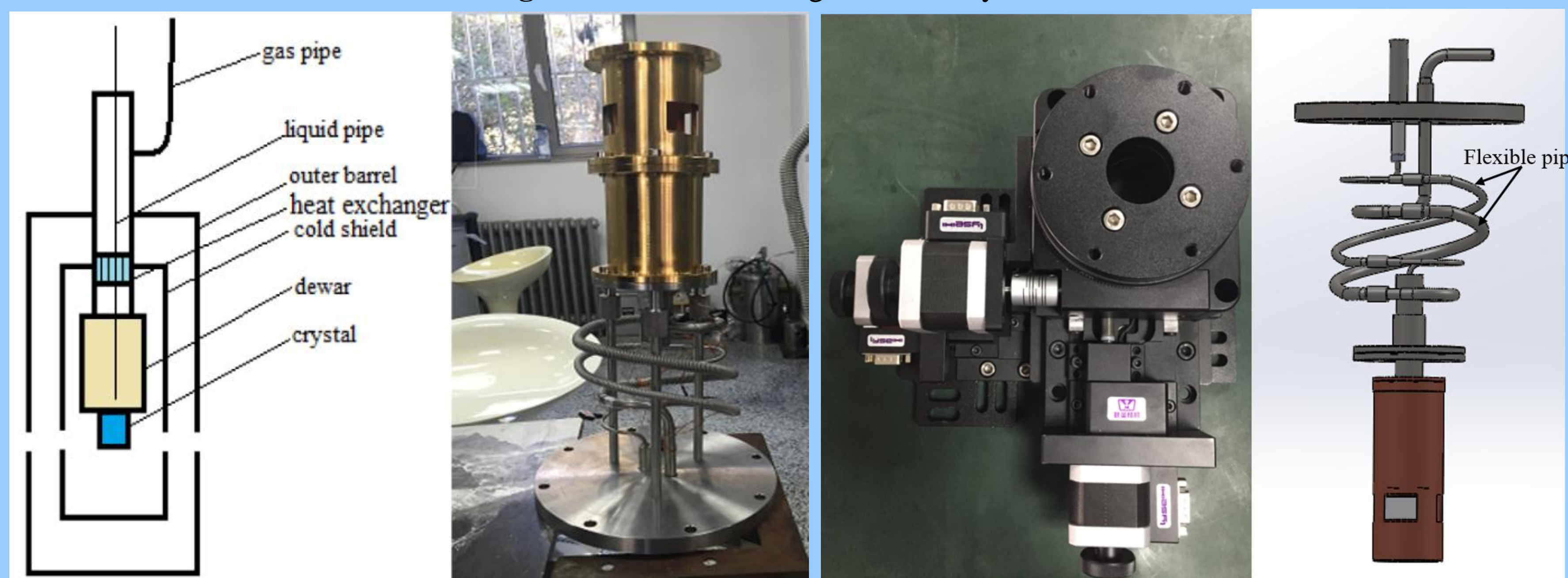
Figure 2. Schematic diagram of the Flexible chamber.
