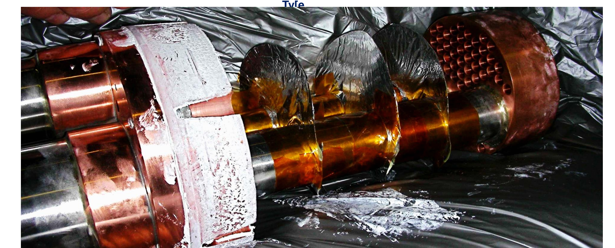
Cryomech PT415 Drop in Cooler 1 st -Stage with a Condenser attached to 2 nd -Stage
