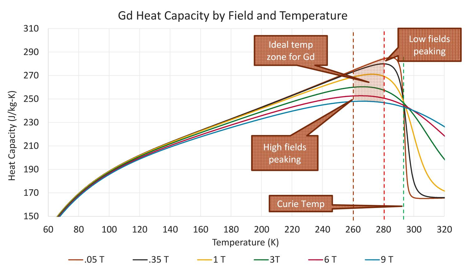
Figure 1: Graph of total heat capacity for Gadolinium showing the magnetocaloric effect driven by field and temperature ranges
