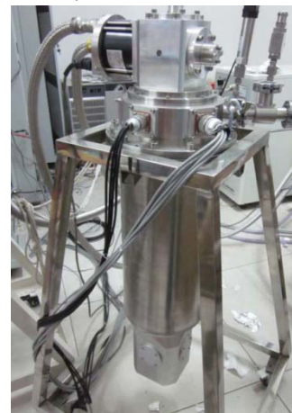
Figure 11. Schematic diagram of cryogenic system Figure 12. Cryostat with a GM cryocooler
