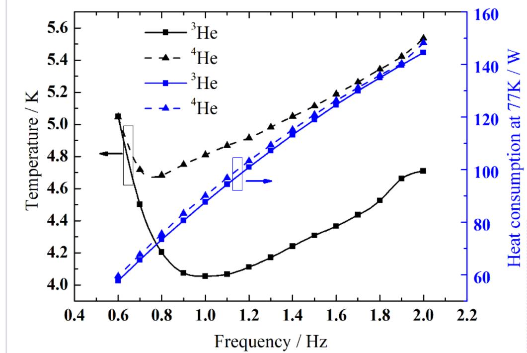
Using <sup>3</sup>He obtains the lowest 4.68K with 50mW load at 0.8Hz while  ${}^{3}\text{He} \geqslant {}^{2.2}_{2.0}$ get the lowest 4.06K with 50mW \\ \geq \text{1.8} load at 1.0Hz. Overall, using <sup>3</sup>He provides lower temperature than <sup>4</sup>He with similar input power.
