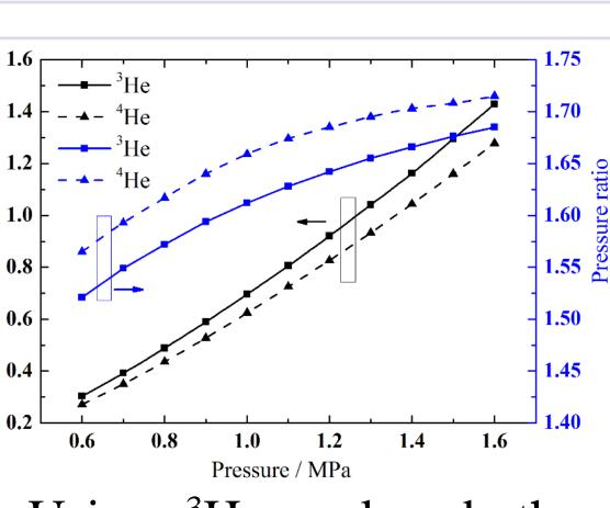
Using <sup>3</sup>He makes both lower pressure ratio and large enthalpy flow out of PT regenerator than <sup>4</sup>He with the change of working pressure.
