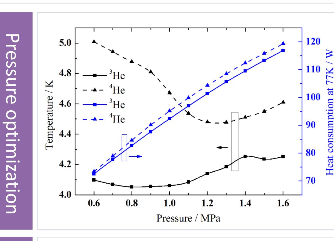
studied at 1.0Hz. Quite similar with influence of working frequency, the \frac{1}{29} 0.8 100 to heat consumption of using two fluids at 77K are similar. The optimal pressure of <sup>3</sup>He is around 0.8-0.9MPa, lower than that of <sup>4</sup>He, around 1.2-1.3MPa. At the optimal pressure, the usage of <sup>3</sup>He is about 0.0038kg in this system, equivalent to 30L gas under STP.
