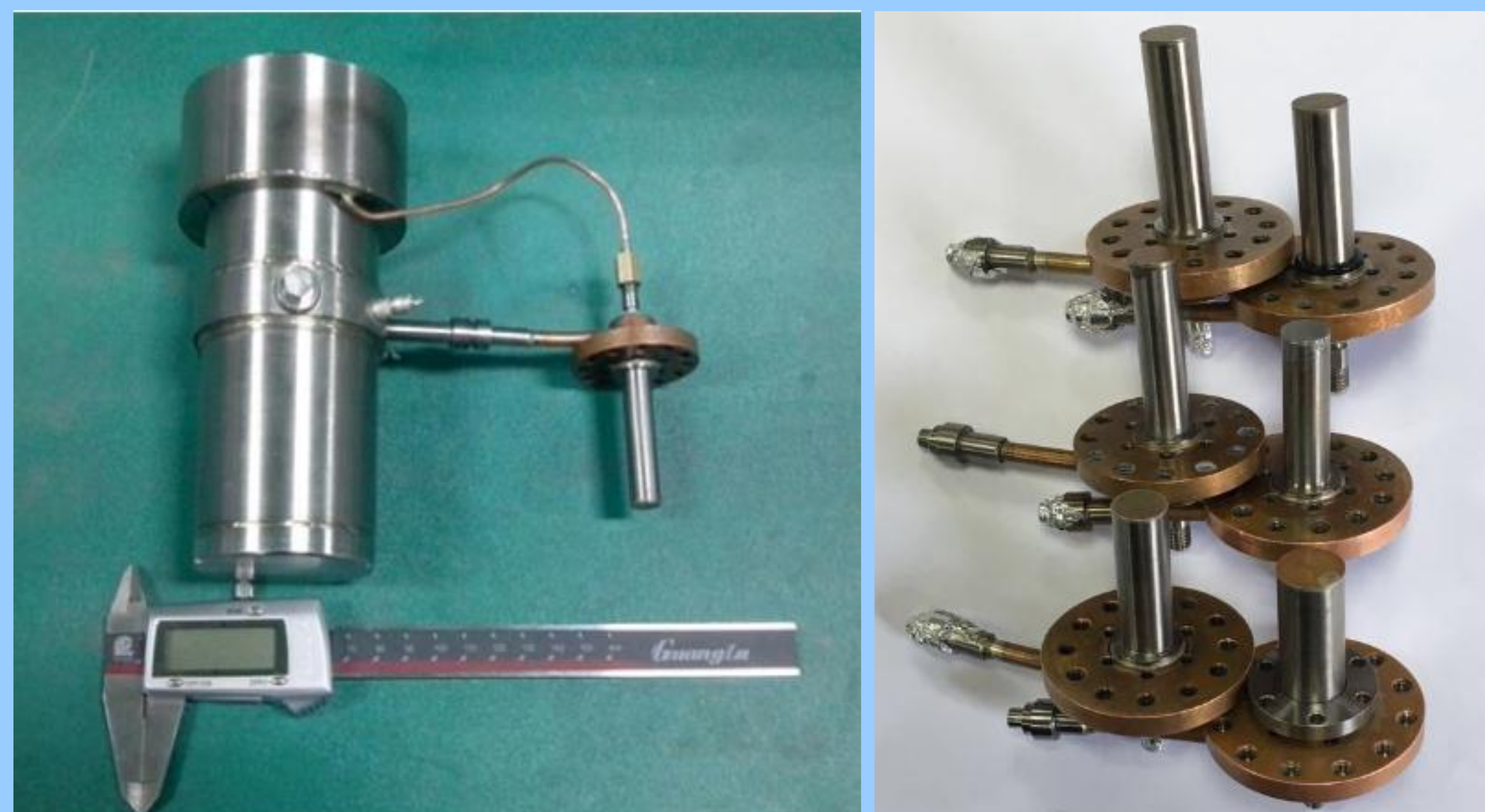
Fig.1 High-frequency miniature pulse tube cryocooler (<2 kg) and six different coaxial cold fingers
