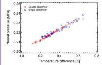
Both of the single and double condenser results follows the same curve. That is, even if the heat transfer area changed, the relationship between the internal pressure and temperature difference did not change. Given ΔT, the internal pressure can be predicted.
