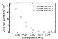
The liquid neon quantity follows the same curve even if we changed the condenser operating temperature.
