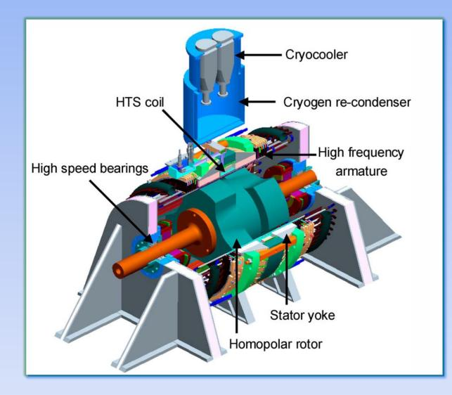
Stationary HTS excitation coil, LNe cooled, BSCCO 2223, Peak field 1 T, 5 MW, 10,000 rpm
