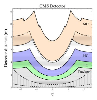
The horizontal (R1) and vertical (R2) hatched areas correspond to optimised regions for DV observations in the muon chambers and tracker respectively
