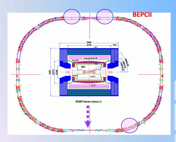
The BEPCII has achieved the designed luminosity  $1 \times 10^{33}$  cm<sup>-2</sup>s<sup>-1</sup> at Apr. 2016.
