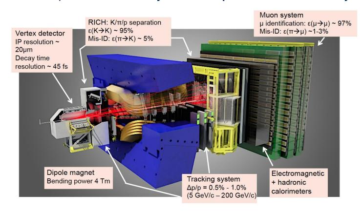
But LHCb is fully instrumented in 2 <  $\eta$  < 5, therefore can serve as a general purpose detector in the forward region
