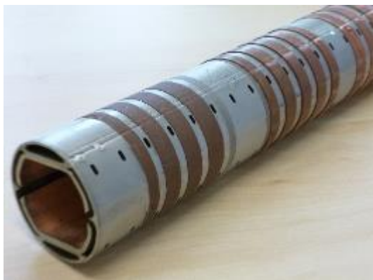
Copper cold sprayed strips on beam screen short prototype
