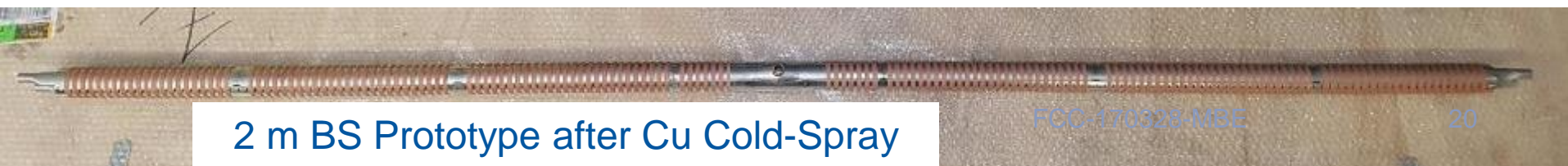
Copper cold sprayed strips on beam screen short prototype
