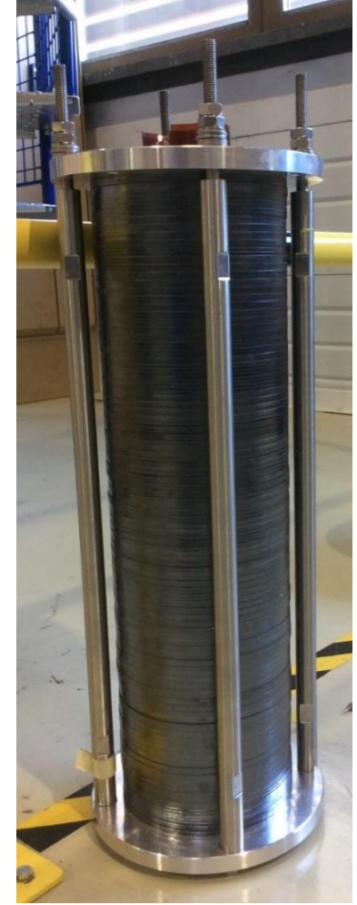
Magnet inside the magnetic laminated yoke
