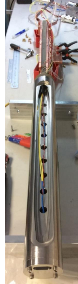
Magnet inside the magnetic laminated yoke
