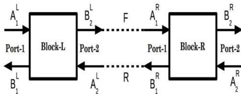
$$S_{11}^{LR} = S_{11}^L + S_{12}^L [I - S_{11}^R S_{22}^L]^{-1} S_{12}^R S_{21}^L$$
