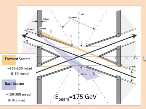
Corresponding SR photon angles estimation for studies of detector SR tolerances (A. Kolano)
