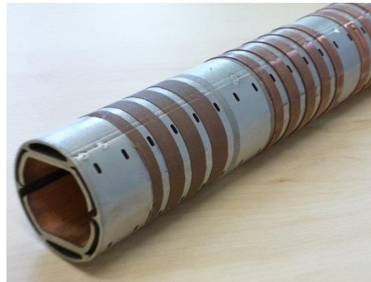
Copper cold sprayed strips on beam screen short prototype
