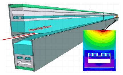
Peak-Energy deposition higher in high-Z absorber blocks of the lower jaws due to higher exposure to secondary showers from first two jaws
