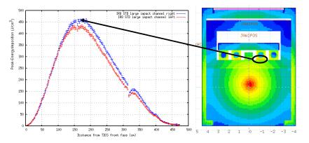
Maximal temperature increase in cooling pipes (CuNiFeMn): ~130 K
