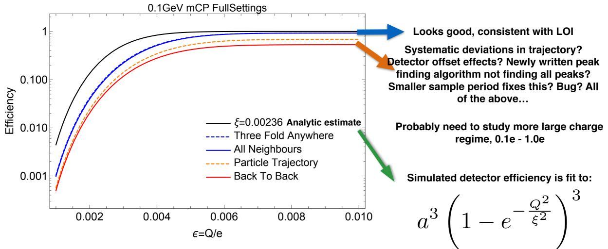
0.00236 is obtained from back of envelope calculation Other 4 curves done entirely from waveform output of Geant4
