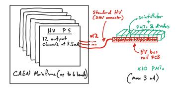
Using CAEN SY55S7LC Mainframe and A7435 HV Boards
