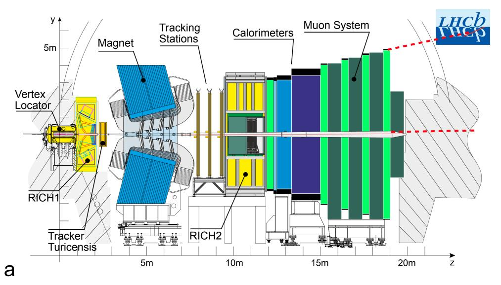
Excellent vertex and IP resolution:  $\sigma(IP) \approx 24 \mu m$  at  $p_T = 2 \text{GeV}$
