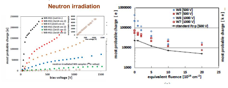
Gain in nonirradiated LGAD achieves 10-20 and goes down under irradiation being about 1
