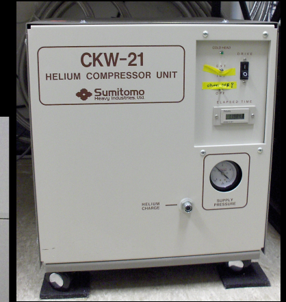
Helium compressor and cryogenerator
