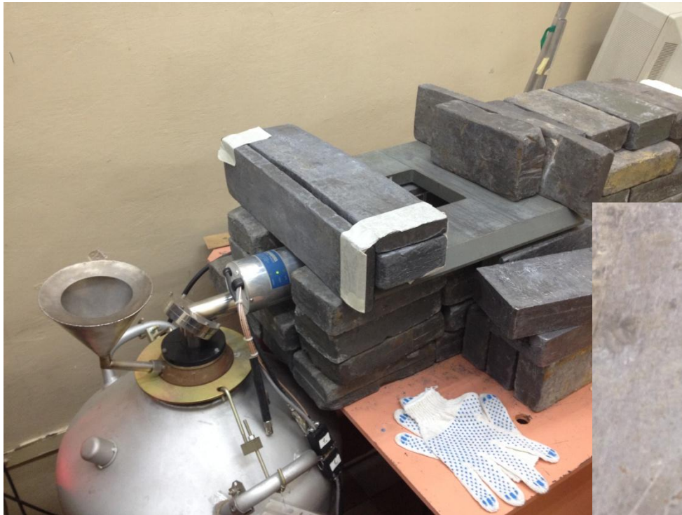
Germanium HPGe detector and leaden cover.
