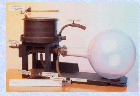
The general procedure was to allow water to evaporate in an enclosed container to the point of saturation and then lower the pressure, producing a over-saturated volume of air. Then the passage of a charged particle would condense the vapor into tiny droplets, producing a visible trail marking the particle's path, their number per unit of length being proportional to the density of ionization (dE/dx).
