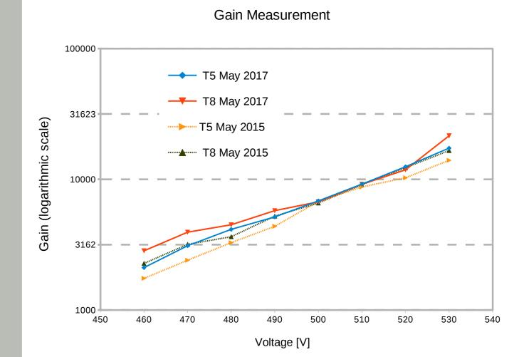
No significant changes on the gain are observed for any of the two chambers  $\rightarrow$  No degradation of the gain due to irradiation observed
