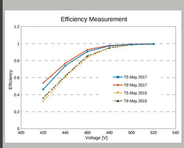
The efficiency is measured with respect to the reference detectors using **muon tracks**
