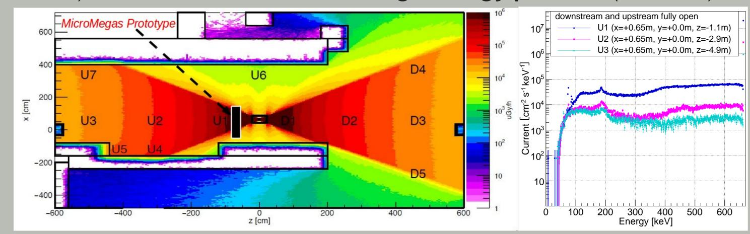
The high source activity, <sup>137</sup>Cs, produces a very intense background gamma field allowing to accumulate doses equivalent to High Luminosity LHC (HL-LHC) experimental conditions in a reasonable time
