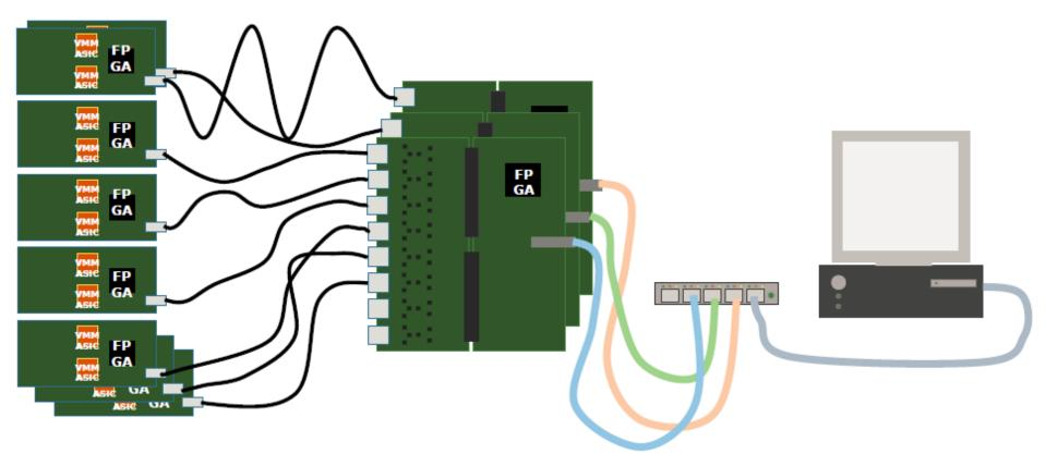
VMM Hybrid  $\rightarrow$  HDMI cable  $\rightarrow$  Adapter card + FEC  $\rightarrow$  Ethernet  $\rightarrow$  Switch  $\rightarrow$ Ethernet  $\rightarrow$  PC
