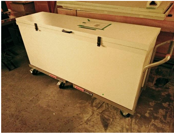
GEM UV tight "fridge" containing one batch of 14 GEM (1.8m x 0.6m max)
