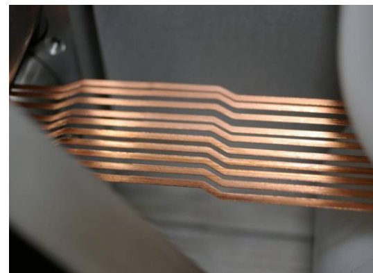
Figure – Cut strands emerging from the punching tool. Ten 2.0 mm strands are formed by continuous punching of 40 mm wide YBCO conductor.
