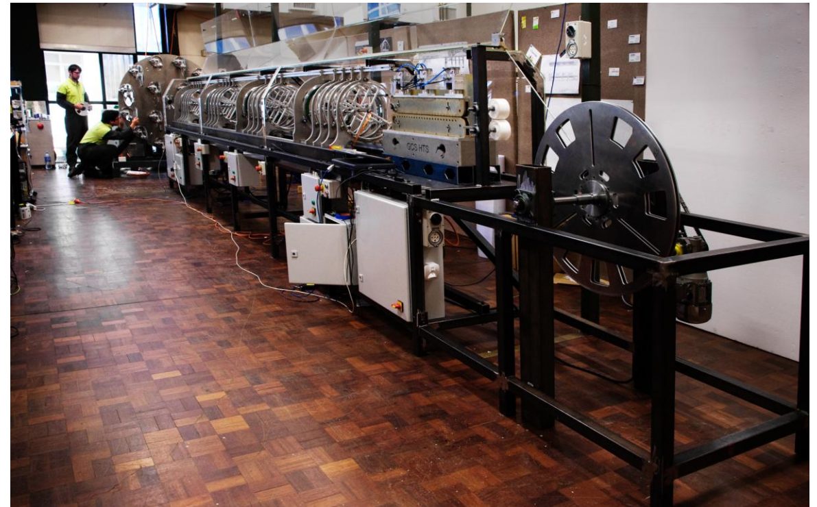
Winding machine for 15/5 cable
