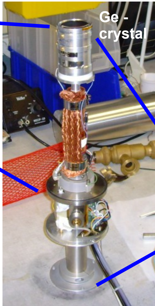
Dismounted endcap for immersion test
