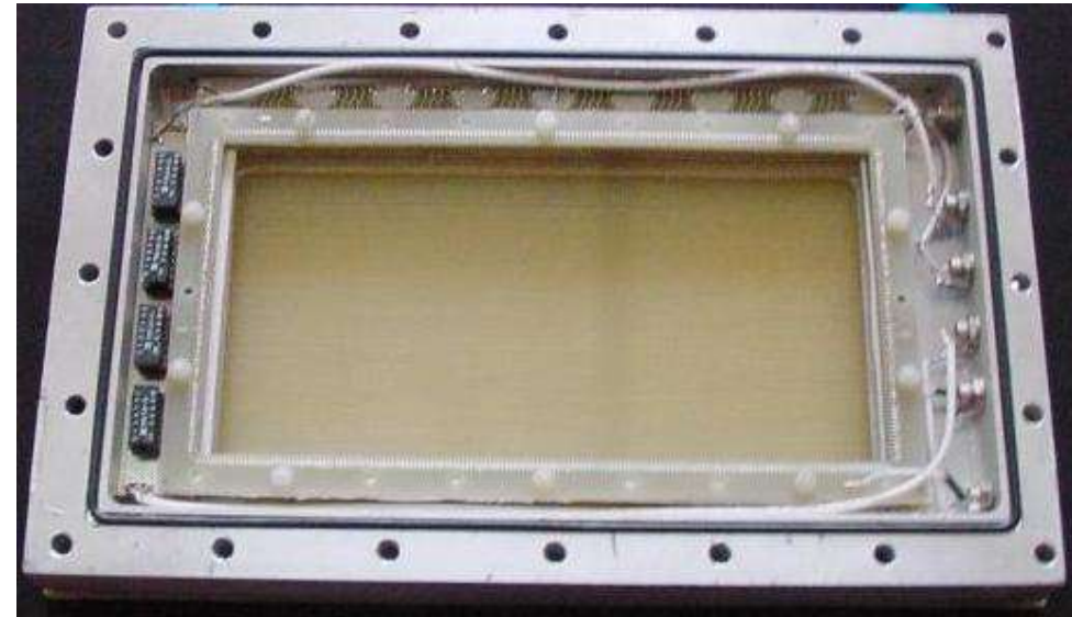
5 electrode, 8"x4", 1.27 mm for GPSC
