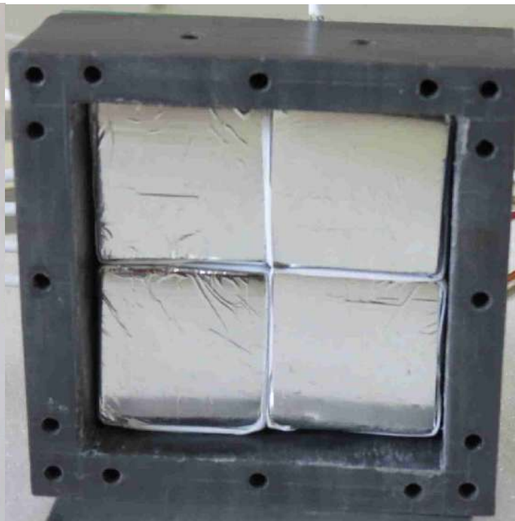
Assembly Config. of CsI coupled to Photo diode
