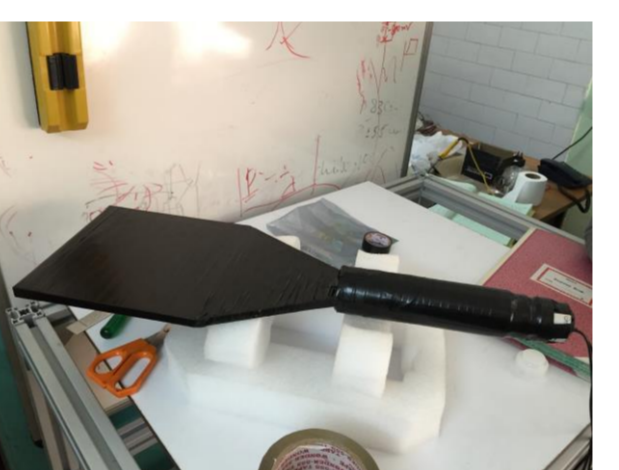
7. Completed Scintillator paddle
