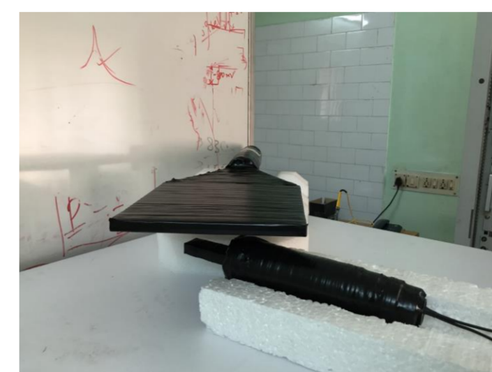
Two scintillators in coincidence
