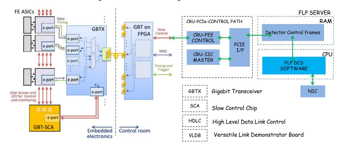
GBT-SCA can only be accessed through GBTX. So, configure the GBTX ASIC first and then interact with GBT-SCA chip when the GBTx is up. The configuration data to be sent is wrapped up in HDLC frame format as per HDLC protocol. As HDLC protocol only defines data link layer. We must add physical layer on top of it. So, HDLC frame is put into GBT frame format and send optically using Gigabit Transceiver(GBT) protocol developed at CERN.
