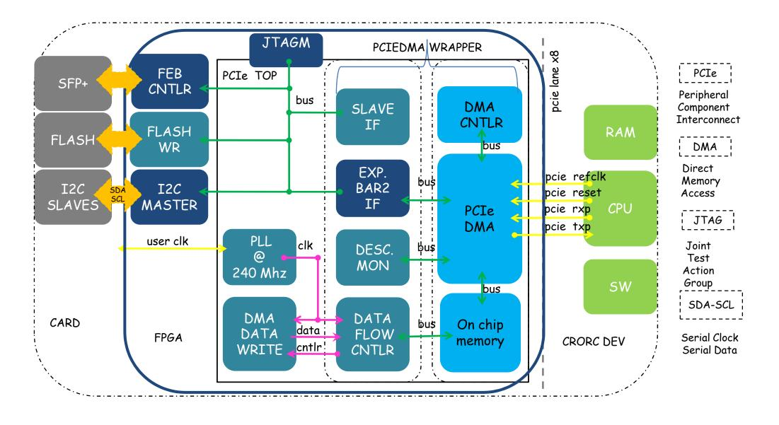
The evaluation PCIe based configuration interface includes FW as well as SW:
