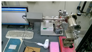
Figure: Portable gas container connected to RGA.
