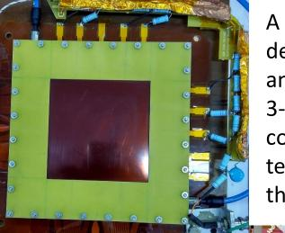
A 10X10  $\text{cm}^2$  triple GEM detector using Ar/CO<sub>2</sub> 70:30 and 90:10 gas mixture, with 3-2-2-2 mm gap configuration, has been tested. The set-up picture of the detector is given below.
