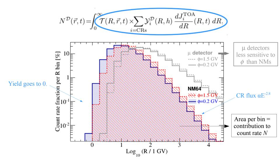
$\rightarrow$  NM64: sensitive to CRs in range 5 GV – 500 GV  $\rightarrow$  Muons detectors: sensitive to CRs in range 10 GV – 1 TeV
