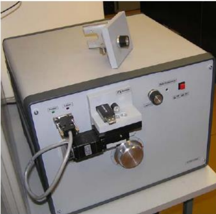
General view of the dosimeter with two-type sample chambers
